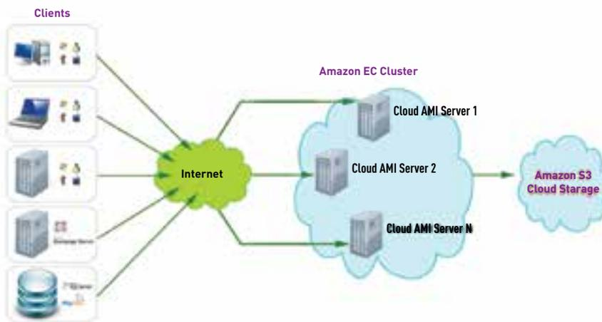
Fig. 2 : Amazon Elastic Compute Cloud Architecture
